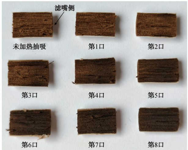
图3 不同抽吸口数对应烟支烟芯段纵切面视图 Fig.3 Longitudinal views of cigarette core segments at different puff numbers
